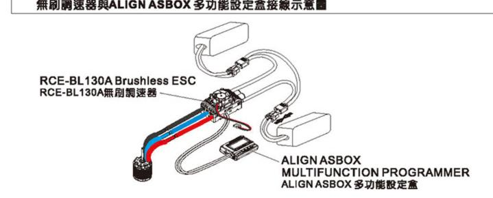
Apply another three-pin wire (with JR male connectors at both ends for connecting ESC and Multifunction Programmer. Plug the three-pin wire into ESC "-+P" port, and also plug into multifunction programmer "ESC" port.
